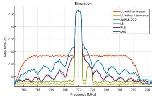
**Fig. 2.** Rejection performance of JWRLS-DCD in full duplex near far scenario.
