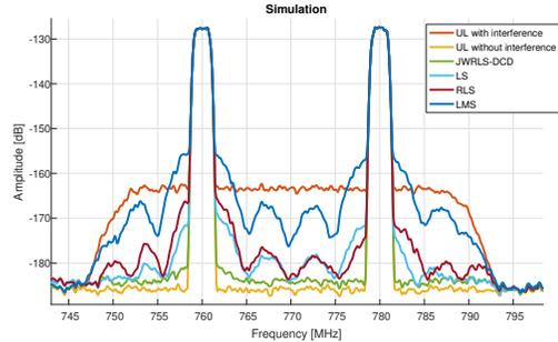
**Fig. 1.** Rejection performance of JWRLS-DCD for two narrow-band UL with wide-band DL in full duplex.
