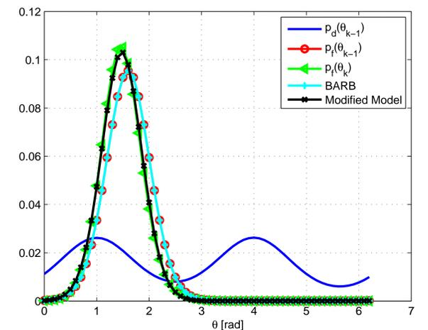
The new algorithm has a negligible loss with respect to DP algorithm while BARB demonstrates a high error floor.
