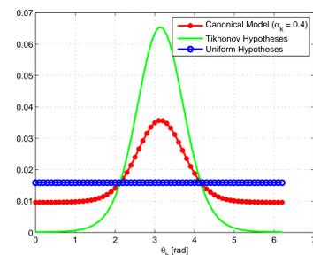
When pilots are available, the uniform distribution helps regain tracking after phase slip.
