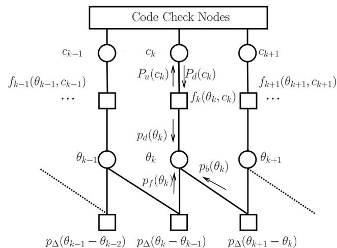
Phase noise SPA messages are continuous and must be approximated using a canonical model.
